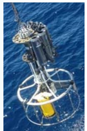
Rosette/CTD/LADCP structure used on the cruise
