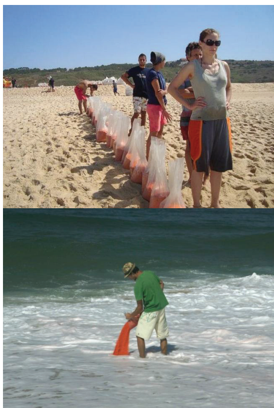
Fig. 6. Injection procedure; (top) injection team ready to carry the tracer 16 kg shots at 30 s interval; (bottom) tracer dumping in the base of the swash zone. This operation lasted 5h and 15 minutes.
