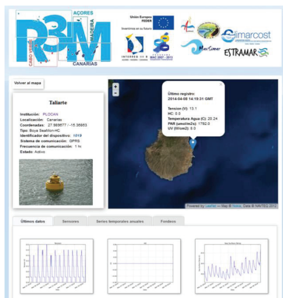
Fig. 5. Screenshot showing real-time information from a moored buoy as example of data display available through R3M portal.
