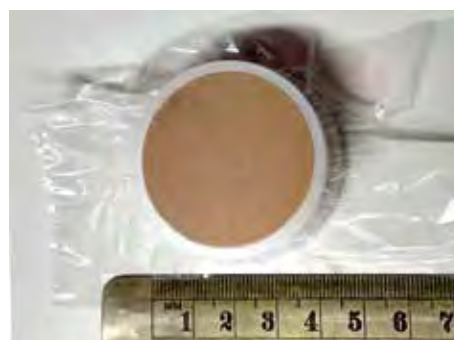
Fig. 6 – Sample cup used to pack the sample grinded powder.
