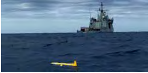
Fig. 5. Glider recovery maneuver from “Meteoro” patrol-boat.
