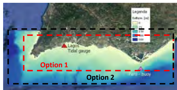
Fig. 1. MOHID Option 1 and 2 model domains and bathymetry. Option 2 domain volume ~5 times greater than Option 1.
