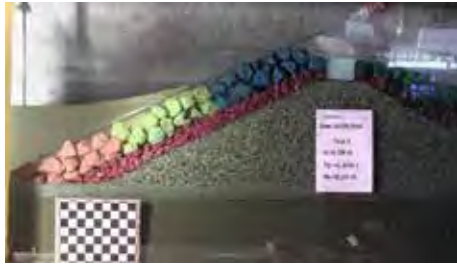
Fig. 1. Model of the breakwater cross-section and experimental equipment setup nearby the structure.
