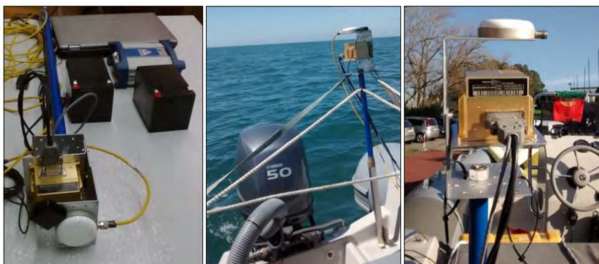
Fig. 2. Global Navigation Satellite System mounted on the survey boat.
