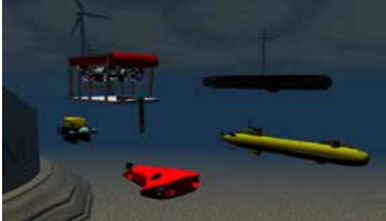
Fig. 5. SWARMS Vehicles presented in the Gazebo simulation environment [RexROV (upper left), IXN AUV by IXION (upper right), SAGA ROV by Desistek (left), Naiad by MDH (bottom) and A9 AUV by ECA (bottom right)].
