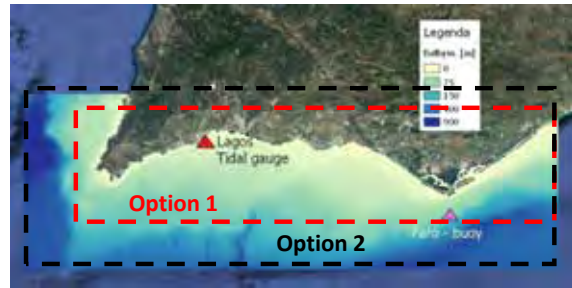
Fig. 1. MOHID Option 1 and 2 model domains and bathymetry. Option 2 domain volume ~5 times greater than Option 1.
