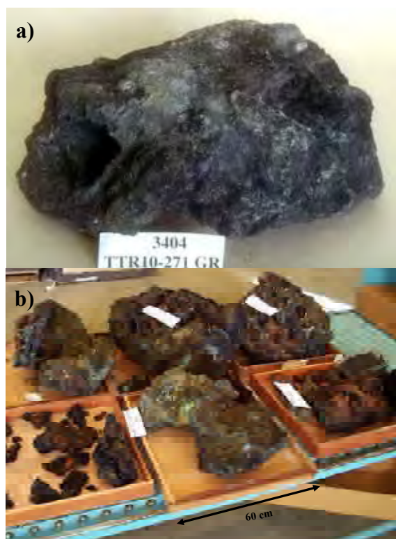
Fig.3. a) Hydrothermal chimney fragment (with a total length of ~60 cm) having a Zn-rich composition showing a well-preserved central conduit. b) A visual aspect of the polymetallic massive sulphide fragments collected in the TTR-10-272-GR sample station.
