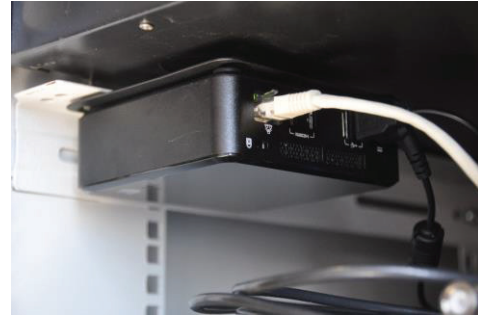
Fig. 3. The compact NUC computer installed in the control room.
