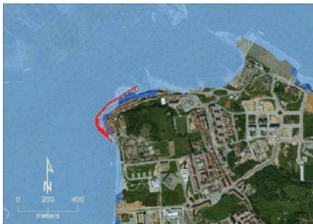
Fig. 2. February 2010 flooding event in SOCC: reconstruction of the flood extension (red patch); model results for the 2010 event (light blue) with SLR (dark blue) (image: ESRI Aerial Imagery).
