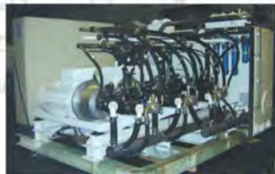
700kW HPU for ship centralized power generation
