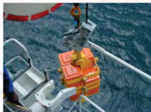
Deployment of a 20m calypso corer Corer, trigger, support fork (RV GO-SARS)
