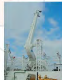
5 T Davit & winch for boat deployment (RV D.CARLOS)
