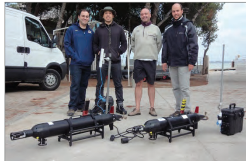
Fig. 5 – Two Seacon AUVs and a Manta Gateway (on the right) from LSTS.
