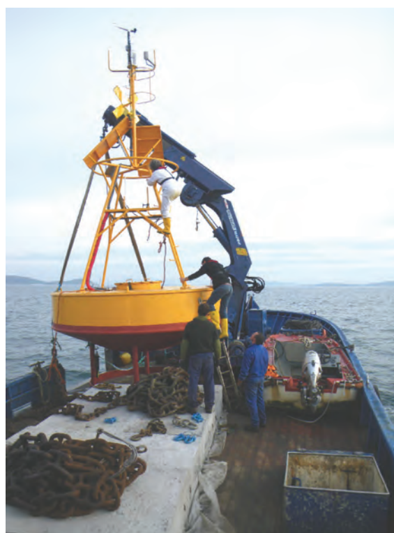
Fig. 3. Mooring maneuver of one of the buoys.
