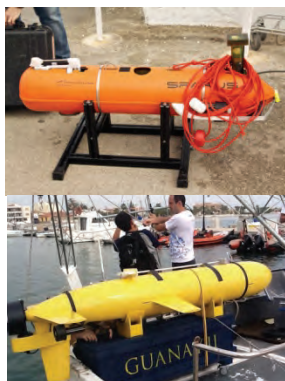
Fig. 3 – Girona University's Sparus AUV (left) and GUANAY II AUV from Catalunya University (right)
