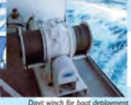
Davit winch for boat deployment (RV MARION DUFRESNE II)
