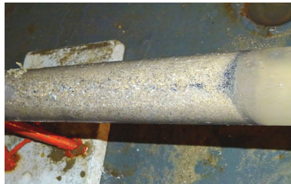
Figure 6. Core sample obtained on the axis of the most active branch of the Nazaré Canyon head. The column is highly homogenous and shows a medium to coarse sand signature.
