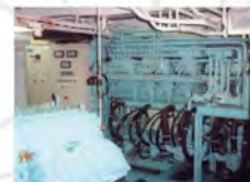
125 kW HPU for winches & A-frame motorization (RV MARION DUFRESNE II)
