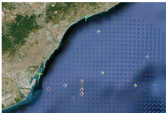
Fig. 8. HF radar surface currents along Barcelona waterfront.
